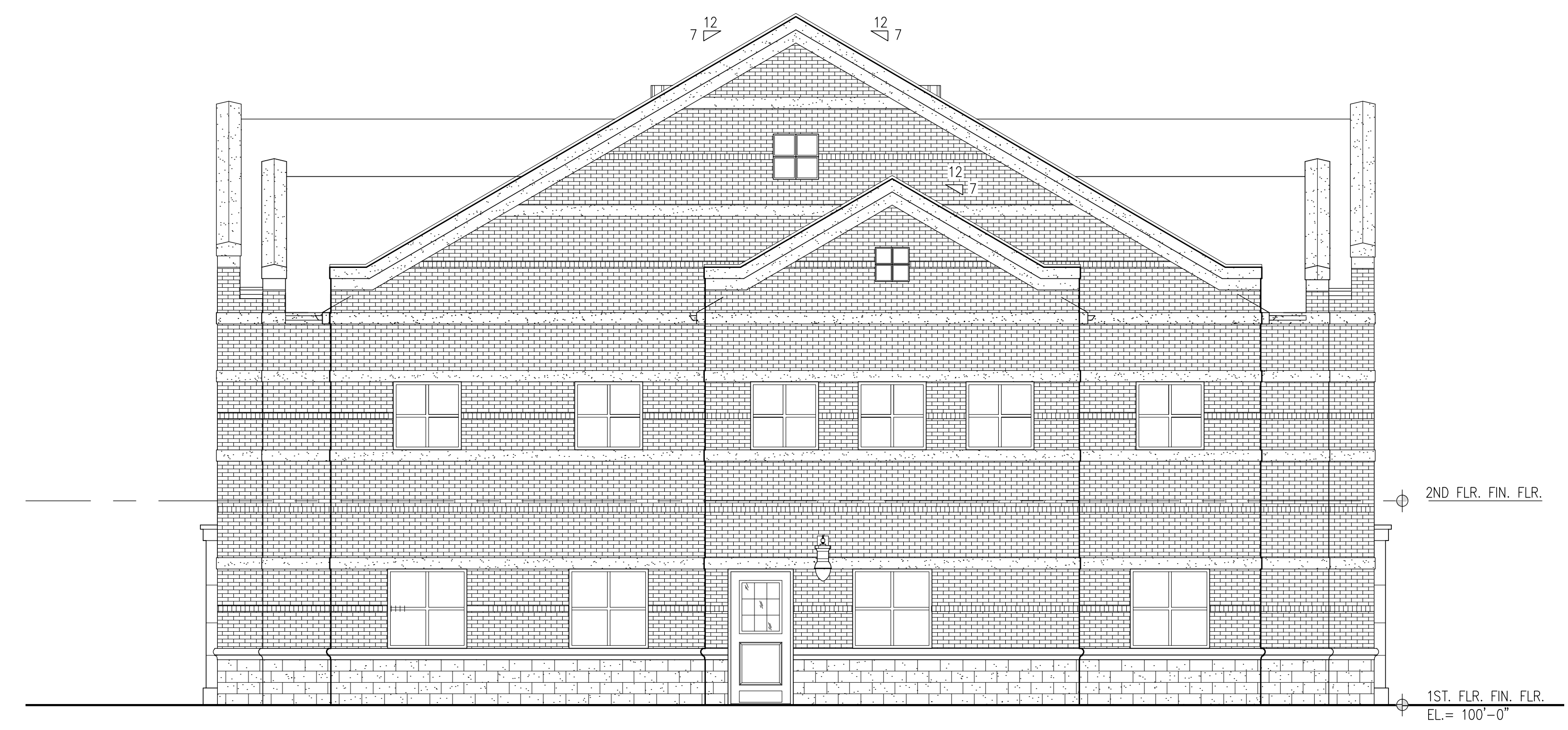
West Elevation (East Elevation Similar) Scale: 3/16" = 1'-0"
