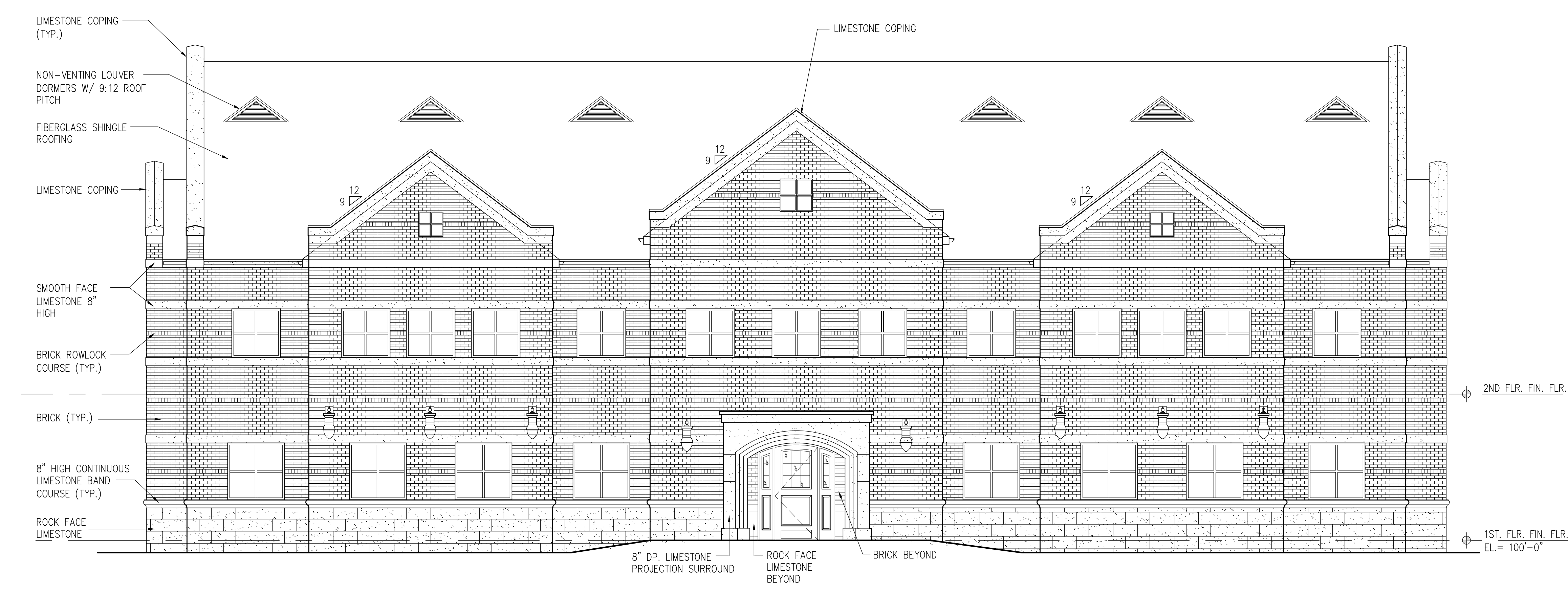
North Elevation (South Elevation Similar) Scale: 3/16" = 1'-0"
